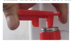
Dispense a cup of water from the hot tap, before plugging into the power socket and turning on the heating and cooling switches on the back. Your cooler is fitted with a child safety hot tap. To operate this tap squeeze the back and front of the red lever together and at the same time push the lever down. It may take up to 30 seconds for the water to flow after installing a new bottle. Be careful as once the heating switch is on, the water will quickly become very hot.
